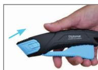
6. Carefully place the front cap to start cutting
