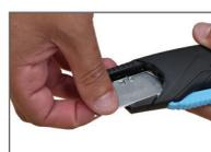
4. Carefully place the blade into position
