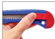
4. Place the blade snapper back into position for use
