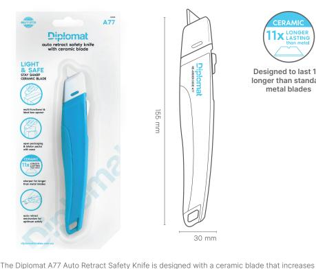
safety while lasting 11x longer than traditional metal blades, which enhances durability and sharpness. This ceramic blade is corrosion-resistant, rustproof, and non-conductive. The safety-focused design includes an automatic retraction feature to minimize injuries
